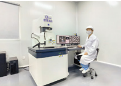
扫描电镜 SEM: Scanning Electron Microscope
