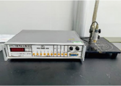
四探针电阻测量系统 Four Probe Resistance Measurement System
