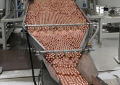
铜球清洗设备 Copper Ball Cleaning Equipment
